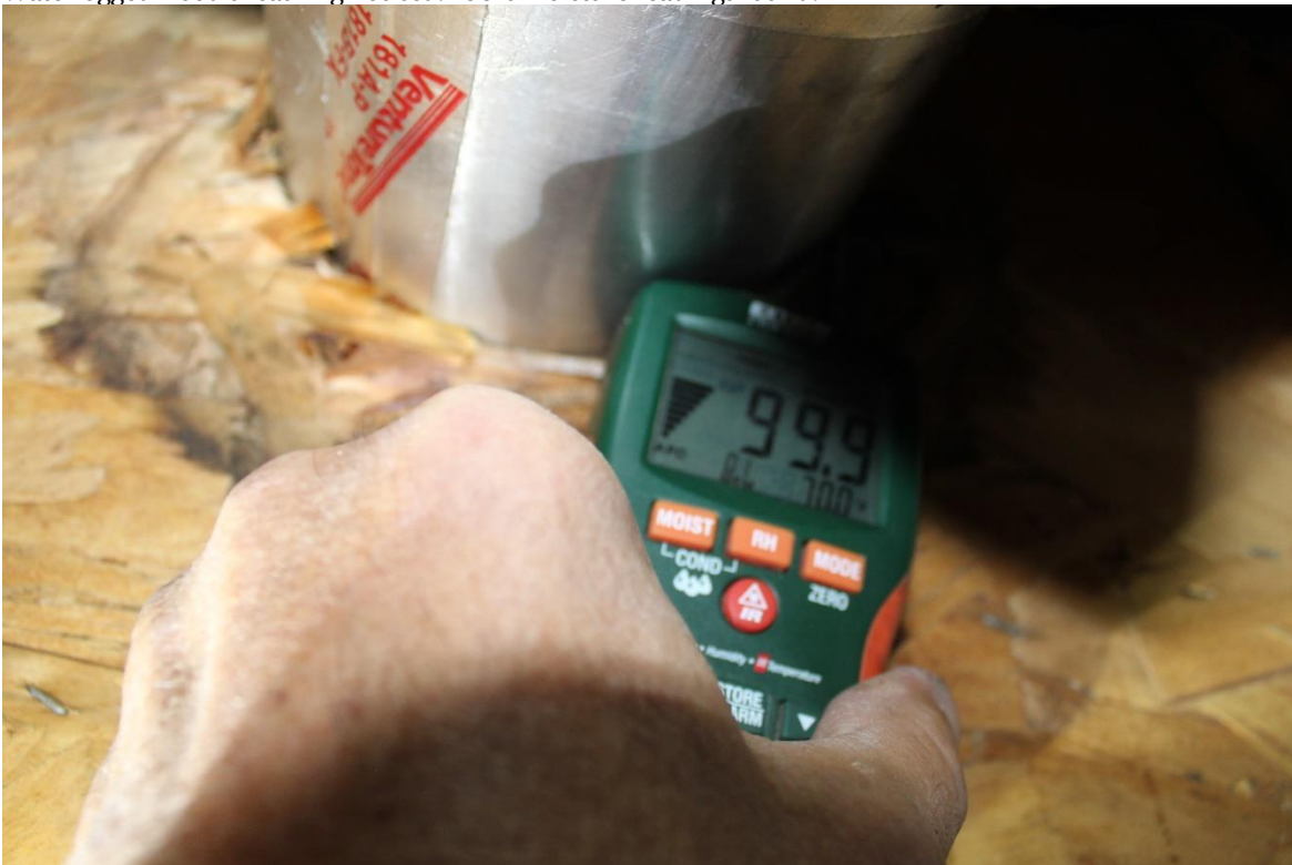
Waterlogged wood sheathing noticed. 100% moisture readings found.
